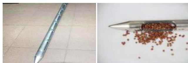
Figure 10. Example of a sampling cup and how it is used
