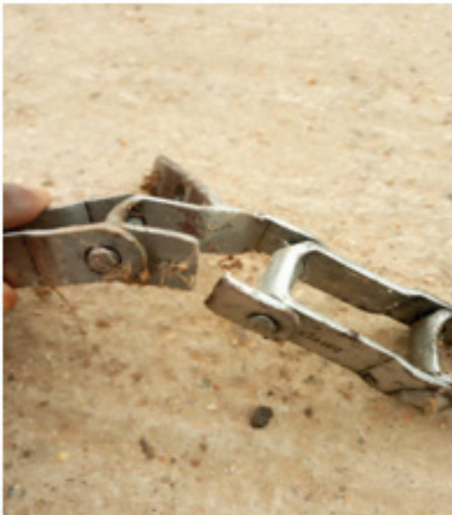
Broken chain conveyor
