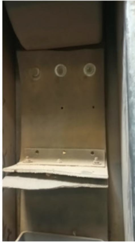
Patched elevator conveyor due to aging
