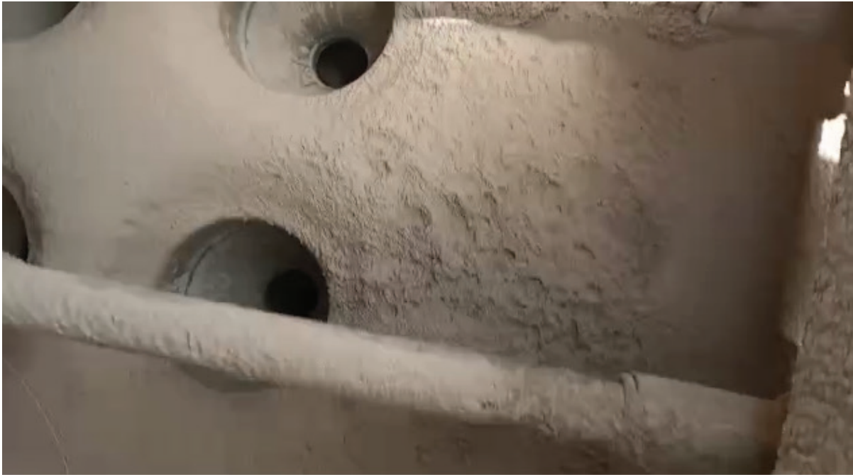
Poor Performance of the Aspirator Showing Accumulation of Grain Dust at Gusau Silo
