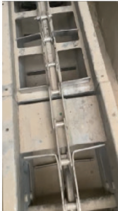
Weak Intake Pit Chain Conveyor failing frequently in operation
