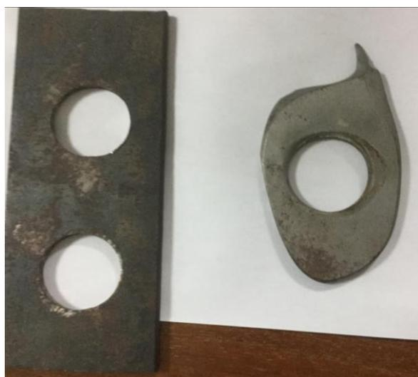
*Figure 1: Left is one of a hammer mill's 48 blades at the start of the day. Right is the blade after a day of milling. The iron residue is most often left in the maize meal. A rough estimate from a miller is that 7 MT of iron shavings are consumed in maize meal each day in Dar es Salaam alone.*
